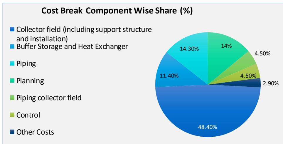
Figure 10: Component wise cost breakdown of a CST system
