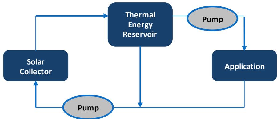
Figure 7: Thermal Storage and control equipment of a CST system
