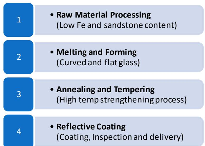
Figure 5: Manufacturing process of solar grade reflectors
