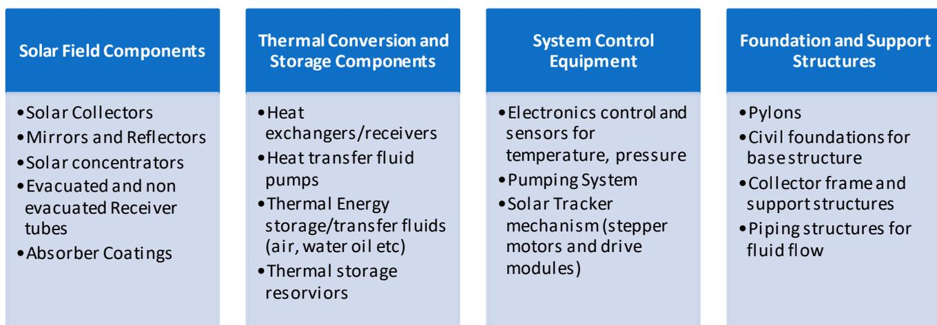
Figure 4: Sub components of a CST System
